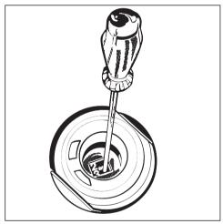
The dosage adjuster in the opening has settings from 1-6 (1-6 ml). It is set to "3" (3 ml) at the factory.
